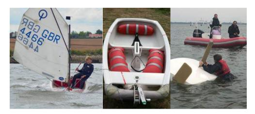
The bags MUST be air-tight, and securely attached to the hull, with at least two 45mm straps (preferably three). Typically, boats will have three sound buoyancy bags of 30 litres capacity for wooden boats or 40 litres capacity for GRP boats or equivalent 'tank' capacity.
