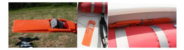
**HINT** – 'Praddles' are the best solution as they can be used with one hand whilst the other hand holds the tiller to steer the boat. They can also be easily stored behind the aft (rear) buoyancy bag tied to one of the bag's retaining straps. (see above). **HINT** When it is not in use keep the lanyard wound around the praddle or tucked away behind the bag so that it cannot become tangled with the mainsheet in the cockpit.
