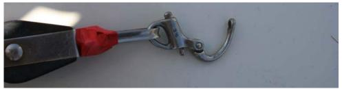
**HINT**- a short-knotted piece of cord attached to the ring on the piston of the snap shackle can really help with an easier grab and operation of the snap shackle. Ensure that this grab cord is not long enough to become caught up in the mainsheet block!
