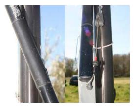
You **SHOULD** ensure that your sprit has protective covering where it touches the mast. (see picture) **WHY?** The sprit and the mast can become worn over time where they rub together. Some sprits come with a protective covering already fitted to prevent
