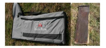
**HINT** The old dagger board on the right is a bit worn on the edges and could reaaly do with some varnish on its edges to stop the water getting into the plywood and delaminating it.
