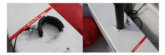
The cord attached to the Mast Lock MUST be attached to the hull at a point level with the top of the thwart. (see picture) . WHY? - this is to show support boat crews that there is a mast lock, so that they can quickly undo the lock and remove the rig quickly if necessary.
