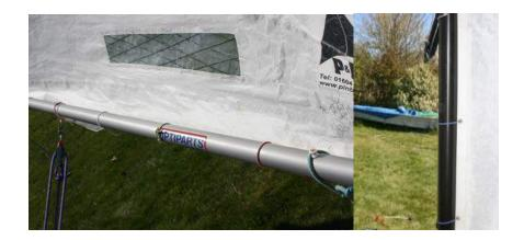
The diagonal tie at the top of the mast is to stop the sail going too far up the mast. The top of the sail **SHOULD** not go past 20mm from the top of the mast. With a more recent sail and mast, the measurement mark on the sail SHOULD be between the 2 measurement marks on the mast. (See picture)
