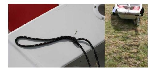
The painter should have a simple loop tied in it 1.5 boat lengths from the bow. It should be tied firmly to an anchor point at the front of the boat. Usually this is the mast step. It should **not** just be tied around the mast or the thwart.
