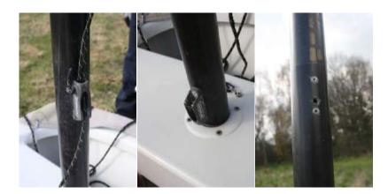
HINT Ideally the mast MUST be able to float without taking in water. If your mast gets water in it, remove it and seal the mast to prevent getting in. (However, note that many of the newer masts do have a deliberate reinforced sealed hole for locating the sprit halyard mechanism). If your mast has lots of old holes from previous fittings, try to seal them with waterproof sealant/filler or use good waterproof tape as a temporary measure.
