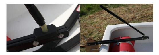
**HINT** - an extension with a rubber joint **SHOULD** not be stored for long periods attached to the tiller and bent against the tiller - this results in cracks in the rubber, and this will eventually lead to its failure.
