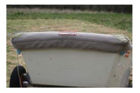
A bow bumper MUST be fitted to a beginner's boat, as this reduces damage to the boat and to other boats. (see above). HINT - after a good knock or two, the foam in the bumper fails and the foam should be replaced (pipe insulation foam can be used as a replacement). Bow bumpers can be purchased from good chandlers including the online ones.
