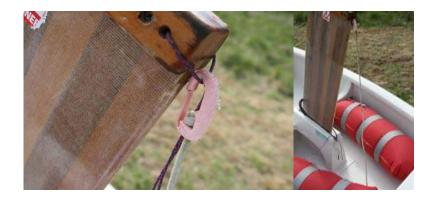
When on the water, the board **MUST** be attached to the boat, using a lanyard (rope) which has a safety hook on the end of it. (See above). This hooks onto a fixing on the boat. **WHY?** This stops the dagger board from being lost in the event of a capsize. The lanyard **MUST** be long enough to enable the dagger board to be inserted and lifted out completely for launching and when coming ashore.
