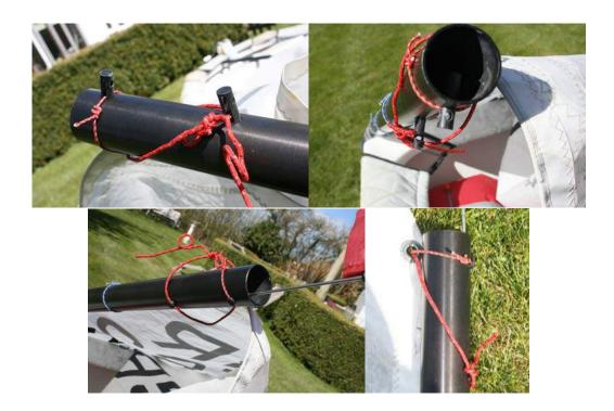
**HINT** More modern sails have the sail ties set in loops at just the right size to slip the sail on the mast after the Sprit halyard has been removed and the kicker released
