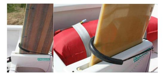
**HINT**- a piece of plastic tube on the elastic where it holds the aft edge of the board stops the elastic being pulled into the case and jamming the board. It can also help the elastic to grip the board and stop the elastic from wearing out. (See above)
