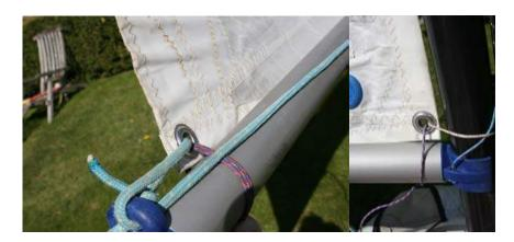
The ties through the remaining eyelets **SHOULD** be of thin cord, holding the sail edge just less than 10mm from the spars, so that the sail can easily move round the spars.
