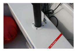
**HINT** If the mast is loose in the mast hole in the thwart it may need a new sleave to ensure that the fitting is sufficiently firm.
