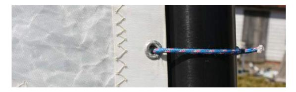
The sail **MUST** be tied to the spars through all the eyelets. The corner ties **SHOULD** be of thin, strong cord; these ties should be tied tightly to hold the sail so that its edge just touches the spars.
